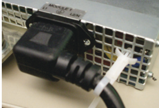
Figure 18: AC Cord Strain Relief for IRU Shelves
