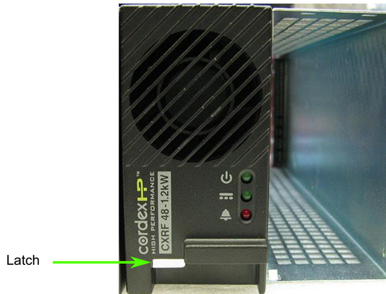
Figure 14: Removing a Rectifier from the Shelf
